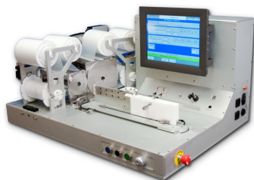
MLL2001 used on balloon pleating/folding machine
