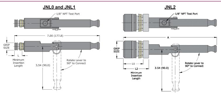
JNL0 and JNL1 - Lever Actuated Connectors for Internal Tubes / Bores
