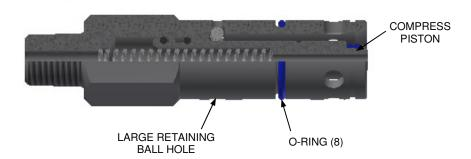
8. Install the sleeve friction o-ring(8) into groove on outside of the body(1).
