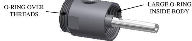
2. Install o-rings into inner piston, making sure that o-rings and back-up rings are located as shown. **NOTE; CUSTOM BACK-UP RING ON BODY SIZE 1 CONNECTORS.**
