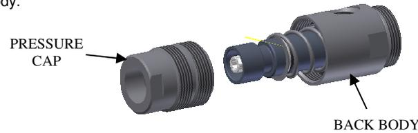
6. Remove inner piston and spring from back body. Discard spring. Remove all o-rings and back-up rings from inner piston and discard.
