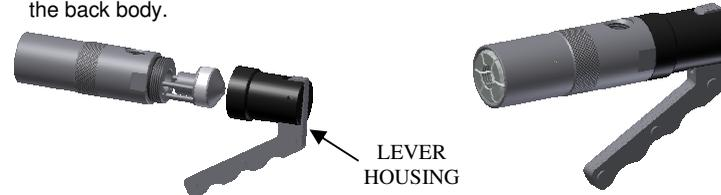
10. With the **Thumb Valve Connector** you just thread the valve housing onto the back body.
