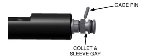
12. Rotate the lever to actuate connector. Visually verify that the connectors gripping and sealing action is correct before introduction of pressurized test media.
