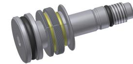
5. Install complete collet and retaining o-ring assembly onto shaft (A) as shown in diagram. Note that the I.D. of the collet assembly is tapered. Larger end of this tapered I.D. goes on the shaft (A) first.
