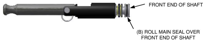
2. Verify correct size and material of replacement main seal.
