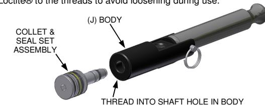
9. Holding body (J) with shaft hole pointed downward, insert threaded end of shaft (A) into hole in body (J). Using a hex wrench in hex hole at front of shaft, tighten shaft into body until snug. Collet set should be threaded in so that edge of collet (F) overlaps edge of sleeve ramp (C) by approximately .02".
