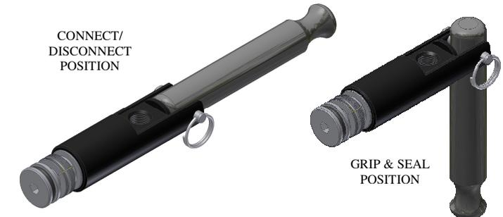
*NuJaws* JNL Connectors provide a reliable leak-tight connection that grips and seals in holes and ports. Simply place the JNL connector into a port, activate the mechanical gripping and sealing action, then introduce the test media. For vacuum to 1000 psi applications with air, gas, or liquid, *FasTestNuJaws* JNL Connectors provide secure, leak tight sealing for manual connections.
