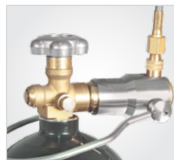
Figure 4c - 4d. Align CGA 580/590 connector tight and square against valve with no visible gap to avoid damage to the sealing surface
