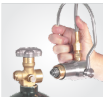
Figure 4c - 4d. Align CGA 580/590 connector tight and square against valve with no visible gap to avoid damage to the sealing surface
