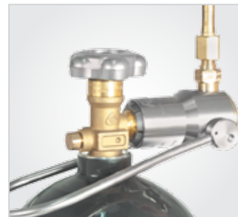
Figure 4a - 4b. Correct CGA 346/540 alignment and connection
