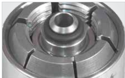
Figure 21. An example of a “good O-ring” main seal.
