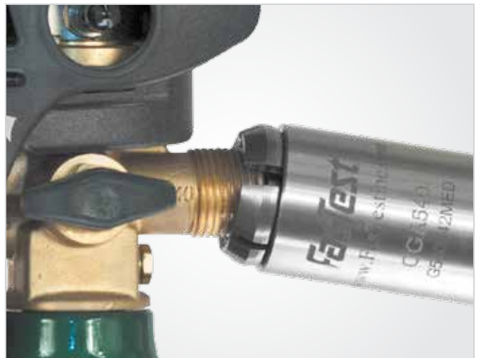
Figure 20. Connector loose and sleeve not forward.
