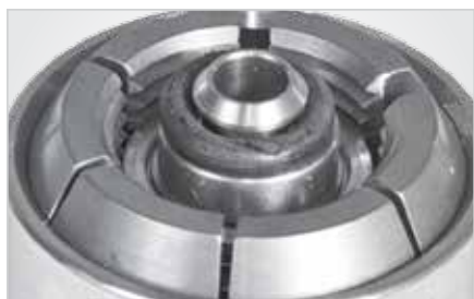
Figure 22. An example of a “bad O-ring” main seal.
