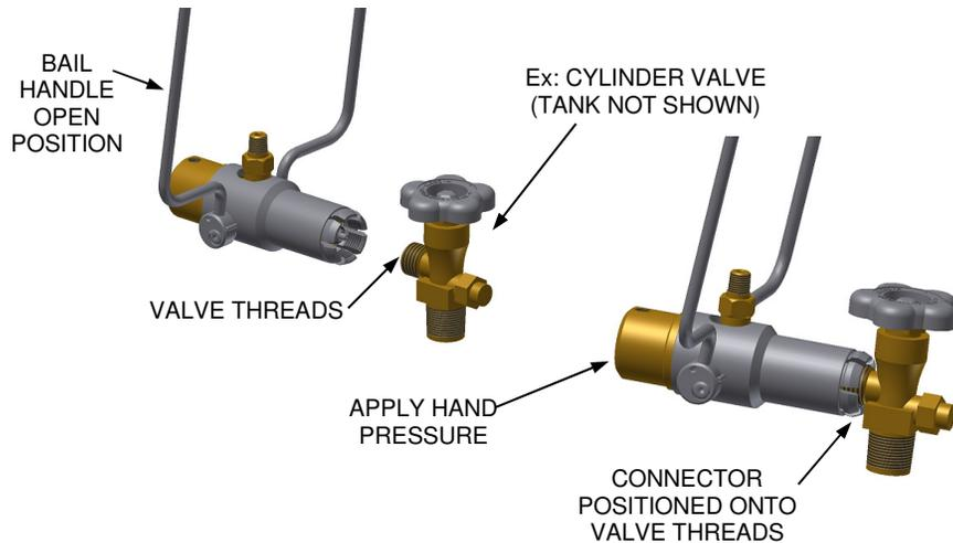
2. Once the *FasTest* connector is over the valve threads, engage the bail handle by rotating the handle down and over the valve. If the bail handle will not engage with relative ease, adjust the pressure to the back of the connector and try again. If the bail still does not engage easily, remove the connector from the cylinder valve and repeat the above steps. Over repeated and constant use, some minor equipment adjustments may be required.
