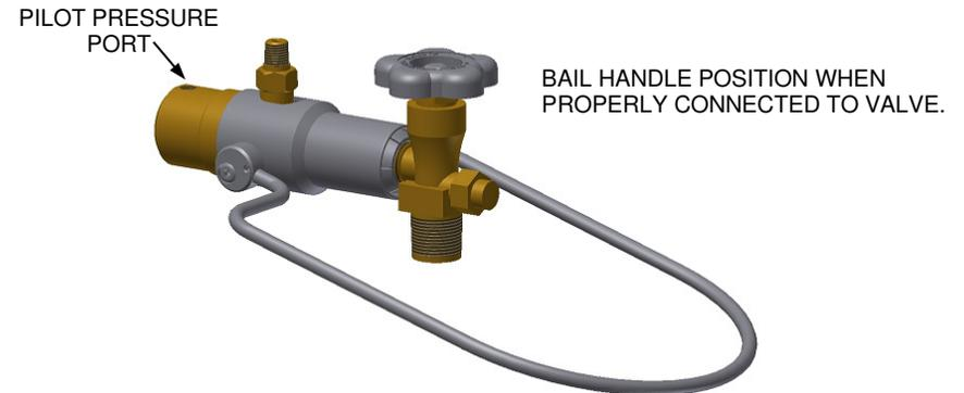
4. Once all cylinders are properly connected, open the toggle valve to supply pneumatic engagement (pilot pressure port) of the connector pin seal. Open the rack vent line and vent residual pressure. (Always follow your company filling procedures.)
