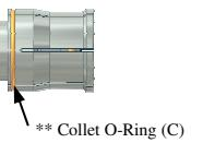
7. After (ZZ) Assy is removed from sleeve grab body with either hand allowing collets to open. Pull Shaft & Piston Assy from collets.
