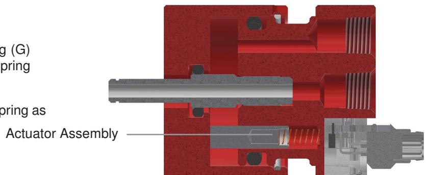
**Figure 11.** Actuator Assembly
