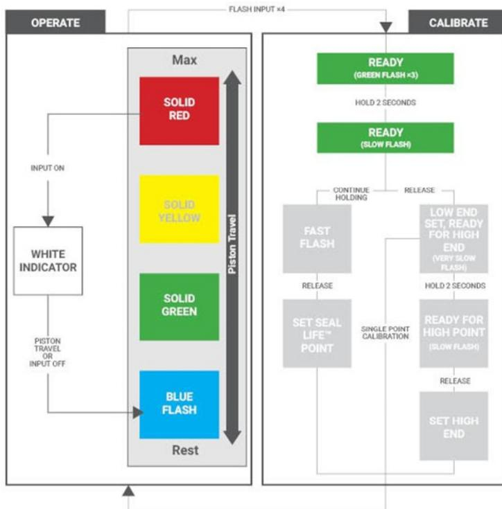
Figure 13. Calibration Flowchart
