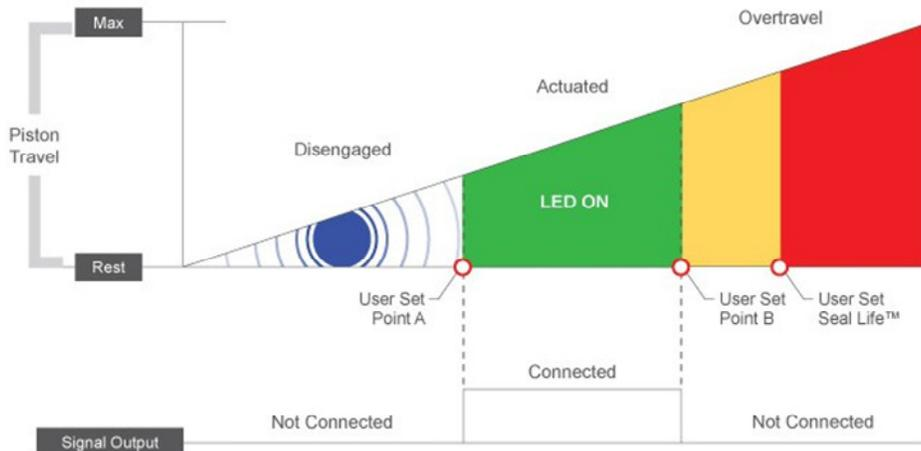
**Figure 12.** Sure Seal™ and Seal Life™ Color Representation
