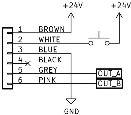
Figure 6A. Solid State Relay Application Electrical Diagram
