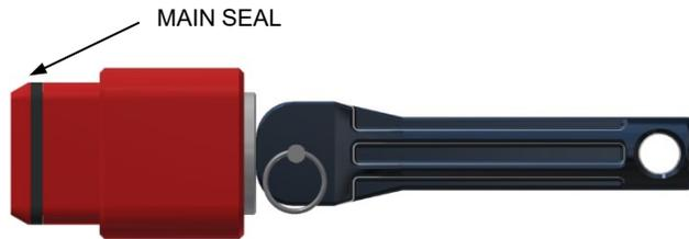
3. Install new main seal using your fingers or a non-marring tool. **DO NOT LUBRICATE NEW SEAL!**
