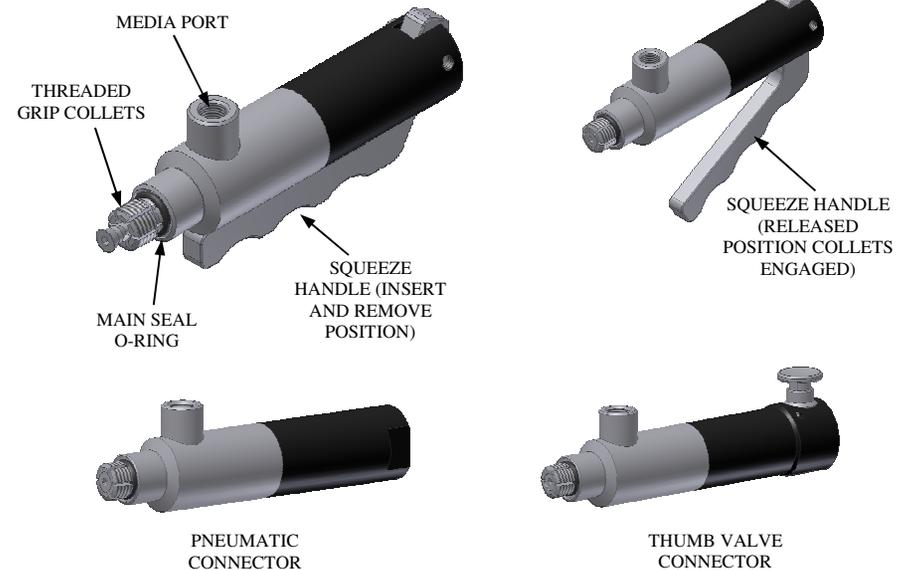
**FasCal/FasMate** Connector provides a reliable leak-tight connection that grips and seals into female threads.
