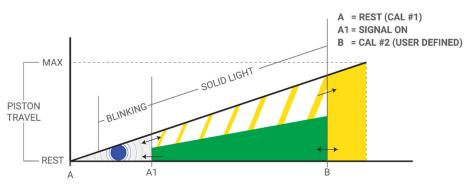
Note: Point A1 is a preset distance from the at rest position (A). As the shaft is extended from rest, it will begin flashing yellow within the good zone. A good connection is only indicated when the shaft retracts from beyond the upper limit (B). If a good connection is made and it's just to the right of Point A1, it could travel through point A1 once test pressure is introduced, and the light will change from green to flashing yellow. Cancel the test, reconnect, and try again.
