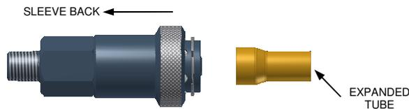
2. Insert tube until it rests against the internal stop.
