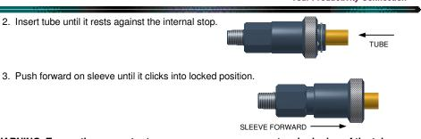
WARNING: Tug on the connector to assure proper engagement and gripping of the tube before introduction of pressurized media.
