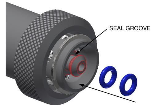
3. When the new seals are in place, they will clearly fit into the groove area. If a portion of the seal is inverted, or can be seen as not being in the groove, use the knobbed end of the pick to assist in pushing the seal into the groove. Be sure the seals are completely seated in the groove.
