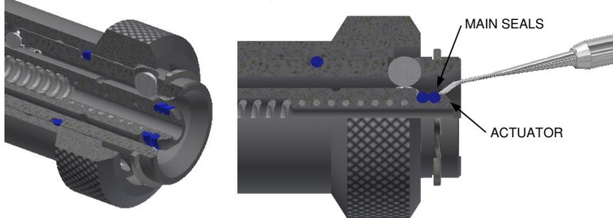
2. Dislodge the main seal and pull it over the actuator tip. Remove the second seal in the same manner.
