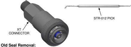
1. Insert the flat end of the STR-012 Repair Pick between the Main Seal and Actuator.
