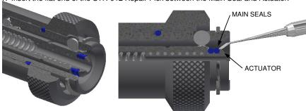
Dislodge the main seal and pull it over the actuator tip. Remove the second seal in the same manner.
