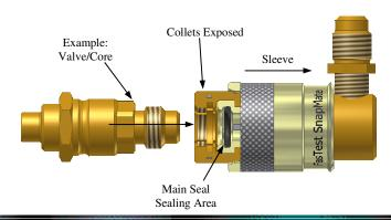
2. Place *SnapMate* collets onto the valve and push the sleeve forward. The sleeve action clamps the collets and opens the internal valves in both the Snap Mate connector and the access valve to allow processing.
