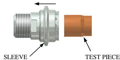
2. Place male end of test piece into the connector and make sure it is completely inserted. Move the sleeve forward to engage the connector into the part.
