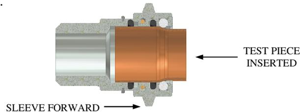
3. Slightly pull the back of the connector to insure engagement before testing. Do not pull back on the sleeve after engagement.
