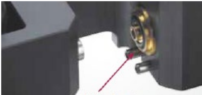
Figure 29. MediMate main seal
