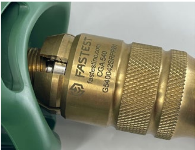
Figure 26. Connector loose and sleeve not forward.
