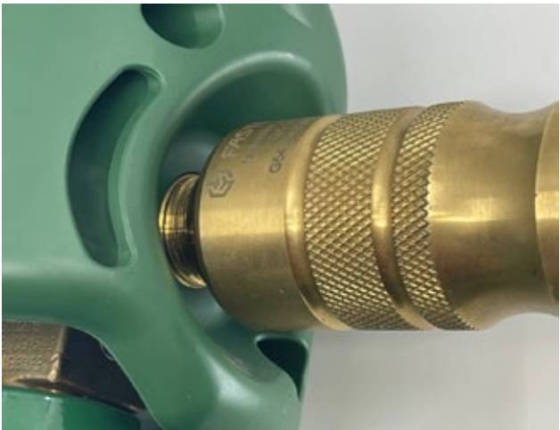
Figure 25. Note excess threads.
