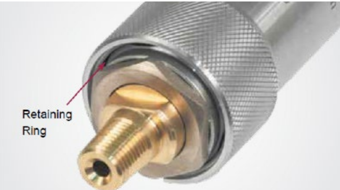
Figure 35. Check retaining ring to make sure it is tightly seated in its groove. ▪ Check internal thread collets for a fixed-center position and even spacing. ▪ An “out-of-round” condition may hinder sleeve operation. A visual inspection of the sleeve is usually sufficient
