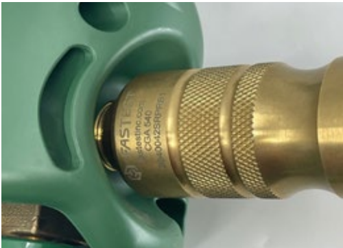
Figure 22. Connector tight to valve
