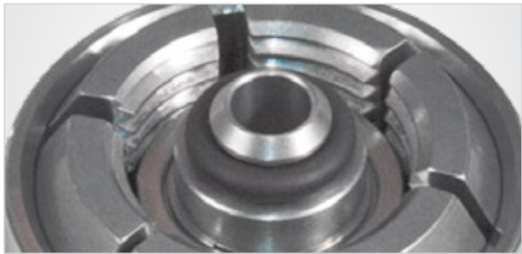
Figure 27. An example of a good O-ring main seal
