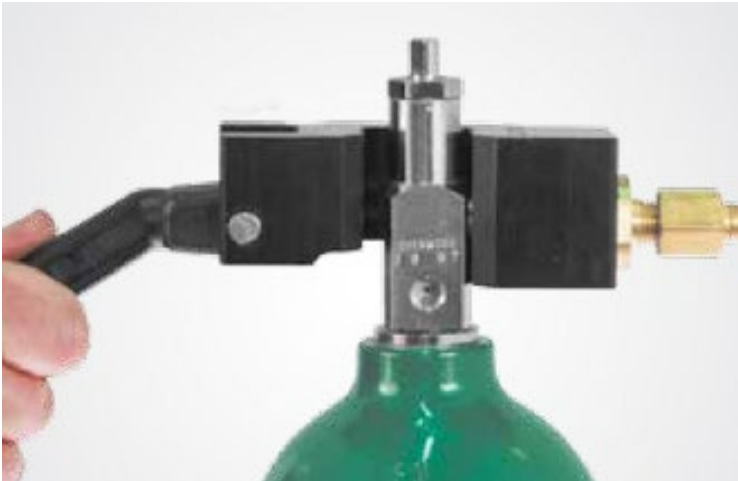
Figure 7. Valve properly aligned.
