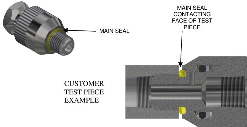
3. Activate test media and perform test. Test pressure will enhance the seal between test piece and Twistmate.
