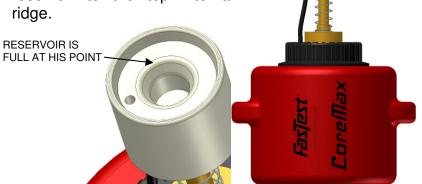
Note the reservoir has a chamfer at the minimum fill height necessary to adequately lubricate the CoreMax core. The oil level must be greater than this line.
