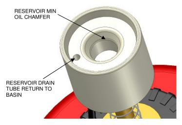
If the reservoir is overfull, there is a return drain tube to return excess oil to the basin.
