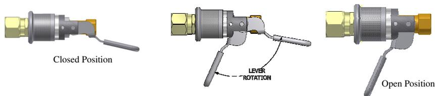
4. **RQD** is now sealed on male fitting and valve is open for flow.
