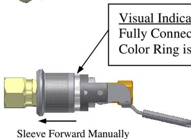
3. Rotate lever on connector.
