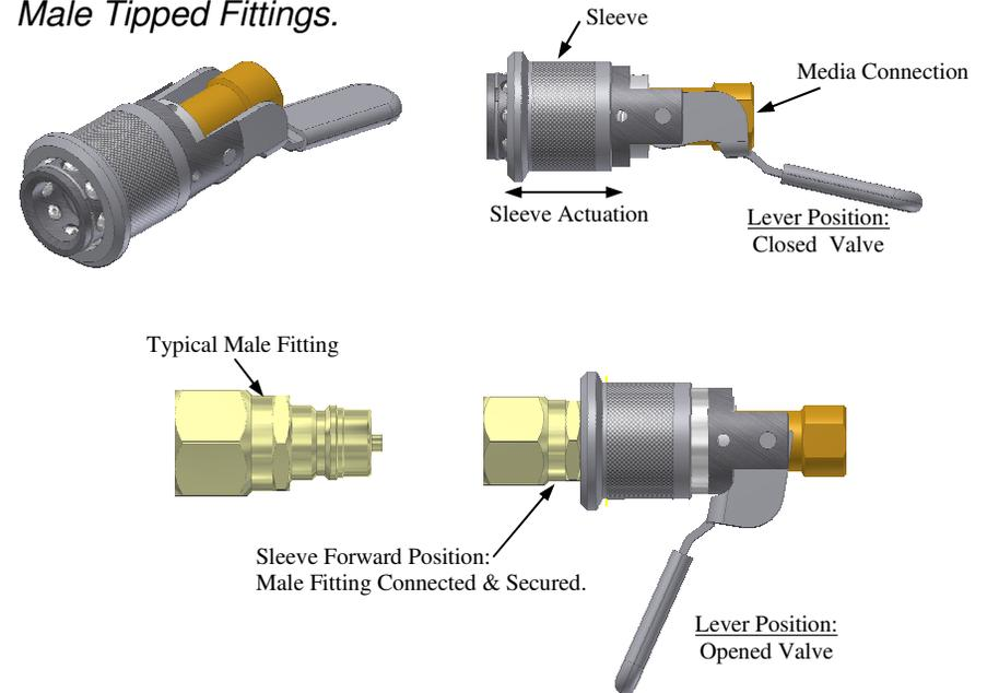
**RQD** Connector provides a reliable leak-tight connection that grips and seals a Male Fitting. Simply insert male end of fitting and slide sleeve forward, gripping balls will secure fitting.
