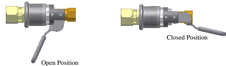
2. Slide sleeve away from male fitting. Visual Indicator will be covered by sleeve.
