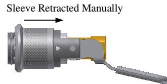
2. Insert test piece and slide sleeve forward collapsing balls around the male fitting.
