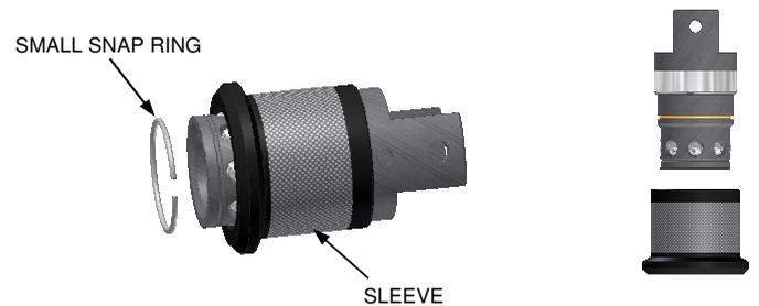
6) Remove the sleeve o-ring.
