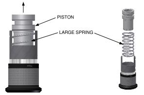
2) Once the brass back piston is removed, remove the spring and poppet assembly.
