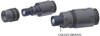
6. Install main seal o-ring, back-up ring and o-ring onto piston. Slide/push piston into inner piston.
