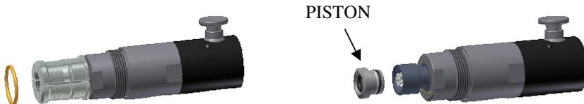
3. Remove main seal from piston, using a sharp pick or some type of like tool, extract main seal from piston AND DISCARD.
