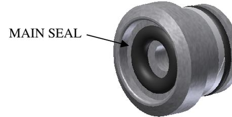
4. Firmly press new main seal into piston groove. Place piston back into inner piston.
