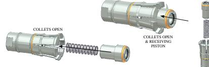
6. With piston down inside collets, hold collets closed with free hand.
