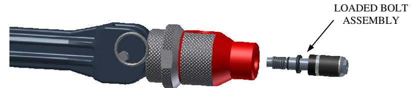
5. Loaded Bolt Assembly threads into an internal shaft. Using same 1/4" wrench or socket. Tighten until you feel a hard stop. Bolt threads into a hard stop inside the internal shaft.
