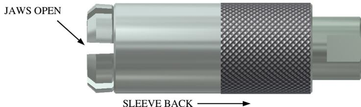
2. Push connector onto formed tube, pushing piston inside jaws. Push far enough to allow bead to be gripped by the jaws.
