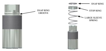
9. Using some type of arbor press or hand tool, press the snap ring into snap ring groove on body. Work press around snap ring until it snaps into groove. When snap ring is properly seated the stop ring will be inside sleeve.
