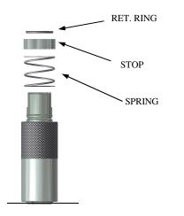
7. Test function before applying pressure to the rebuild connector.
