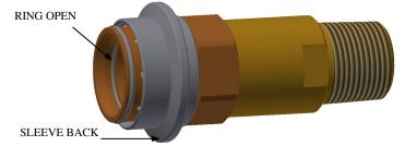
2. Push connector onto relief valve. Push far enough for retaining ring to get past hex of relief valve.
