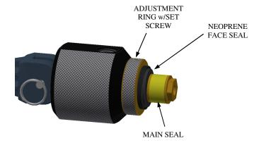
7. Rotate handle 90° degrees in either direction. Main seal is compressed as handle is rotated. This action draws/pulls the test piece into face seal.
