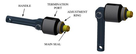
**GZNV** Connectors provide a reliable leak-tight connection that grips threaded ports and seals on port face. Simply insert male end of connector into port and rotate handle to engage seal to port.
