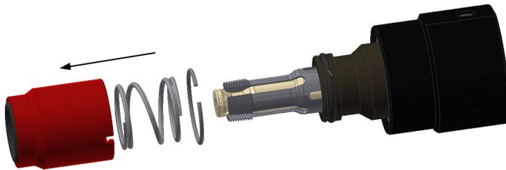
3. Stand the remaining assembly up into a vertical position. Using a sharp pick remove the spiral retaining ring. NOTE: THIS RETAINING RING IS UNDER SPRING FORCE. TO EASE THE REMOVAL OF THIS SPIRAL RETAINING RING USE ARBOR PRESS TO HOLD AND PUSH THE BODY DOWN BEFORE ATTEMPTING TO REMOVE SPIRAL RING.
