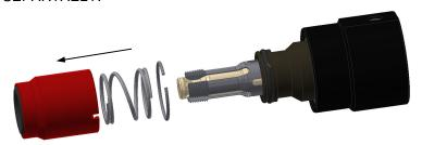
3. Stand the remaining assembly up into a vertical position. Using a sharp pick remove the spiral retaining ring. NOTE: THIS RETAINING RING IS UNDER SPRING FORCE. TO EASE THE REMOVAL OF THIS SPIRAL RETAINING RING USE ARBOR PRESS TO HOLD AND PUSH THE BODY DOWN BEFORE ATTEMPTING TO REMOVE SPIRAL RING.
