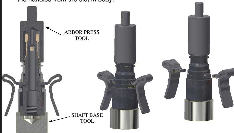
10. Remove shaft from body, push shaft in direction shown. Some pressure will be required because collets have to flex outward to allow shaft to be removed.
