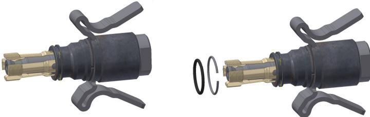
10. Install the new retaining ring onto body just pasted the o-ring groove. Lube new o-ring and install in groove.
