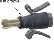
11. Squeeze handles and install new sleeve spring over the relaxed collets.
