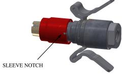
2. ARBOR TOOL EXAMPLE: INSIDE DIAMETER OF THE ARBOR TOOL MUST BE SLIGHTLY LARGER THEN FLEXED COLLETS.
