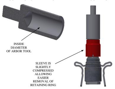
3. Squeeze handles, this will move shaft forward and relax the collets. Remove/pull sleeve and sleeve spring. Discard spring. NOTE: MAIN SEAL KITS ARE SOLD SEPARTAELY.
