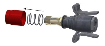
4. Remove and discard o-ring and sleeve retaining ring.
