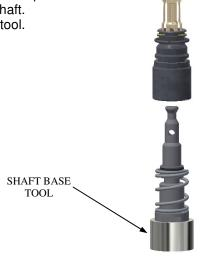
5. The body/collet assembly must be pressed far enough to install handles.
