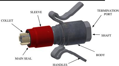
**ZGN** Connectors provide a reliable leak-tight connection that grips female threads and seals on part face. Simply insert male end of connector into threaded port and apply termination pressure.
