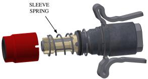
12. Continue to squeeze handles and install sleeve over spring and gently work the sleeve over the body o-ring. NOTE: MAIN SEAL CAN REMAIN IN THE NOSE OF THE SLEEVE DURING THIS INSTALL.
