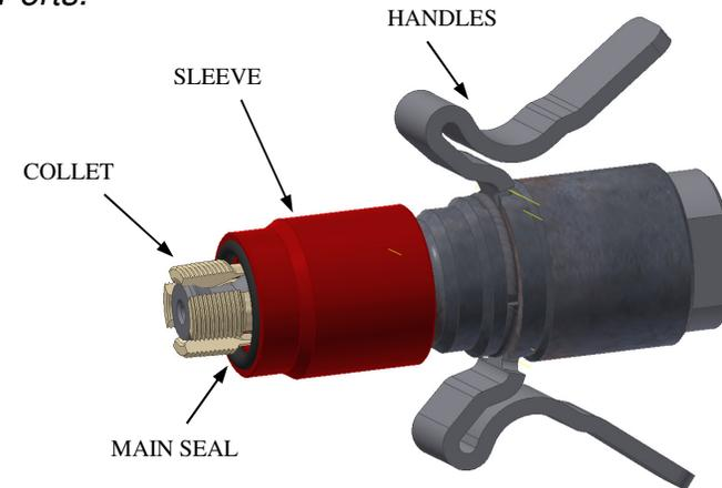
**ZGN** Connectors provide a reliable leak-tight connection that grips female threads and seals on part face. Simply insert male end of connector into threaded port and apply termination pressure.
