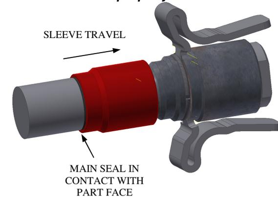
4. Release the handles. Collet will bite into test piece and pull test piece against the main seal.
