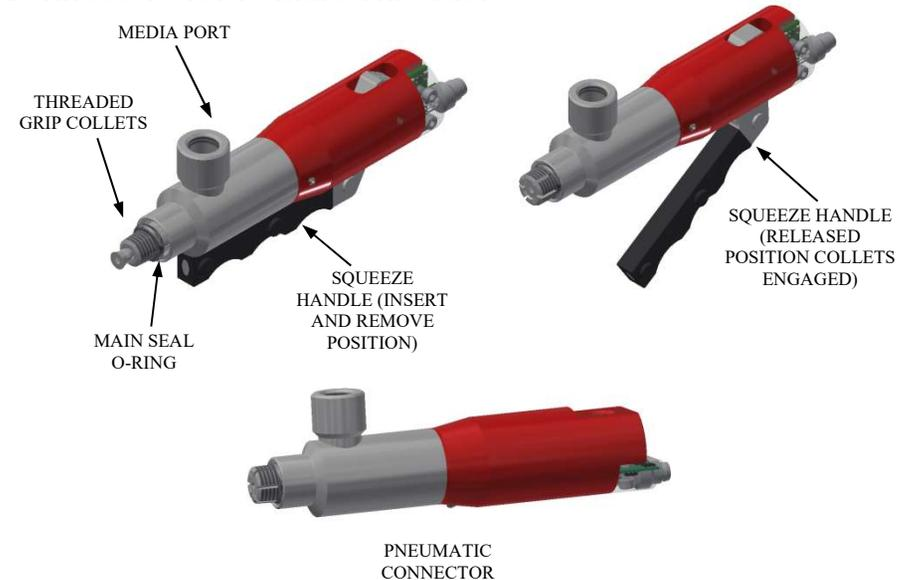
**FasMate** Connector provides a reliable leak-tight connection that grips and seals into female threads.
