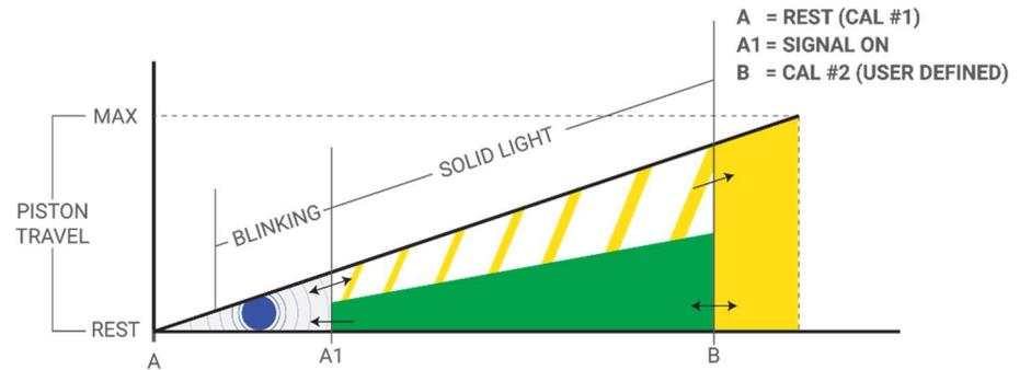
**Note:** Point A1 is a preset distance from the rest position (A). As the shaft is extended from rest, it will begin flashing yellow within the good zone. A good connection is only indicated when the shaft retracts from beyond the upper limit (B). If a good connection is made and it's just to the right of Point A1, it could travel through point A1 once test pressure is introduced, and the light will change from green to flashing yellow. Cancel the test, reconnect, and try again.
