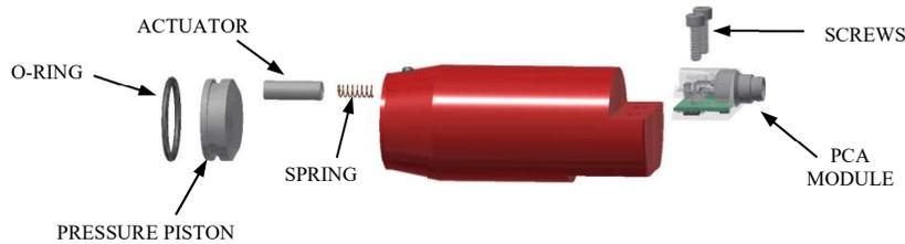
4. Remove o-ring from pressure piston and replace.
