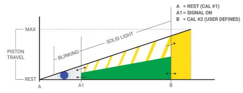
Note: Point A1 is a preset distance from the rest position (A). As the shaft is extended from rest, it will begin flashing yellow within the good zone. A good connection is only indicated when the shaft retracts from beyond the upper limit (B). If a good connection is made and it's just to the right of Point A1, it could travel through point A1 once test pressure is introduced, and the light will change from green to flashing yellow. Cancel the test, reconnect, and try again.
