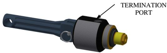
3. Using a 6 point socket or box end 6 point wrench, loosen and remove the front shaft. **Note: Shaft has been secured with Loctite 242 at the factory.**
