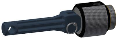
8. Load front shaft with new seal mount, brass washers and remaining used parts.
