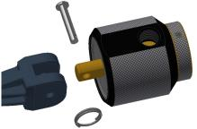
9. Using a small flat screwdriver or like tool, remove spiral retaining ring from body and discard.
