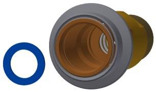
3. Discard old seal and replace with new seal. Carefully push around outer diameter of seal to lock seal into piston. Take care not to damage seal. Using a relief valve to push seal into piston may also work.
