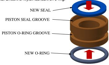
5. Lubricate piston bore with small amount of krytox. Install new spring inside bore and then carefully place piston assembly inside back body bore.
