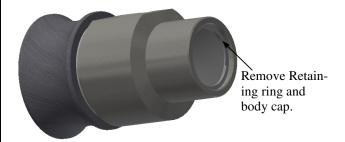
2. Remove and replace the body cap o-ring, lube with refrigerant oil.
