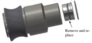
3. Reinstall the body cap retaining ring.
