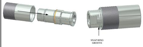
8. Place assembly with collets down on work surface. Using stop ring, push new large sleeve spring down over body, followed by stop ring and the new snap ring.
