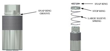
Using some type of arbor press or hand tool, press the snap ring into snap ring groove on body. Work press around snap ring until it snaps into groove. When snap ring is properly seated the stop ring will be inside sleeve.
