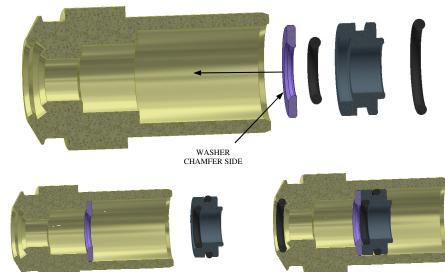
3. Place collets around body, use new collet o-ring to hold collets in place.
