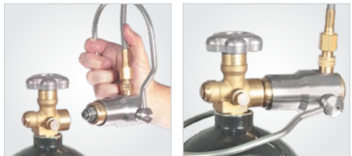
Figure 4c - 4d. Correct alignment and connection of connector for internally threaded valves. Note: align connector tight and square to valve face with no visible gap showing collet threads.
