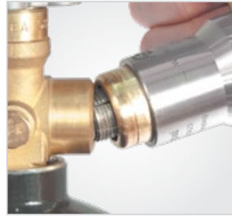
Figure 7c. Misaligned connection with internally threaded cylinder valve.
