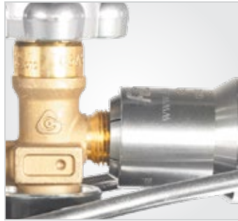
Figure 6d. Exposed threads indicating possible short connection on externally threaded cylinder valve.
