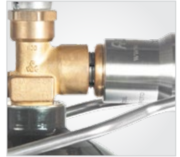
Figure 7d. Exposed threads indicating possible short connection with internally threaded cylinder valve.
