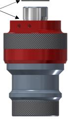
34. Install second actuator/magnet and spring components into hole on backside of the housing.
