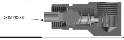
While maintaining compression carefully install depressor ring and begin to thread the piston cap onto piston body. The KA04CMAT connector has a small o-ring that is placed in the thread relief groove of the piston cap.
