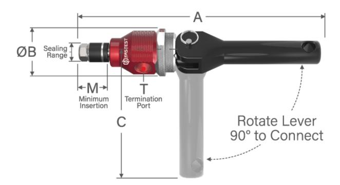
Actuation: LeverPressure Rating: 3.4bar (50psi)Vacuum Rating: VacuumLeak Rate Capability: 1E-5cc/s HeConnection / Application Method: ManualGrip Method: Seal Friction
